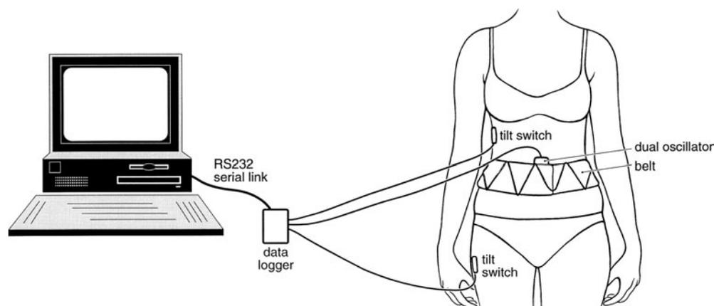
Figure 2. Typical sensor positioning.
