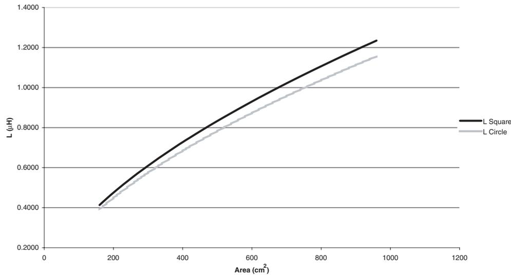
Figure 1. Inductance versus area for curved and non-curved shapes.
