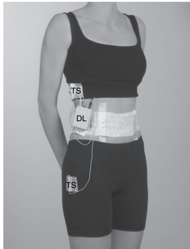
Figure 1. Ambulatory abdominal inductance plethysmography (AIP) equipment in situ . 3, 4 TS, Tilt switch; DL, Data Logger.
